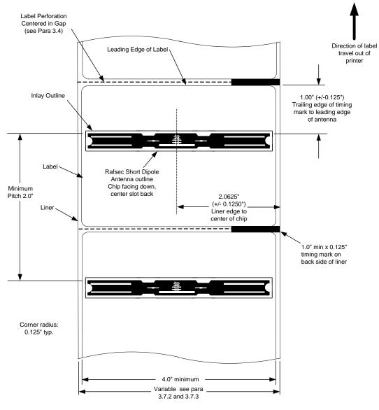
Printronix RFID Label Requirements for Rafsec Short Dipole Inlay
